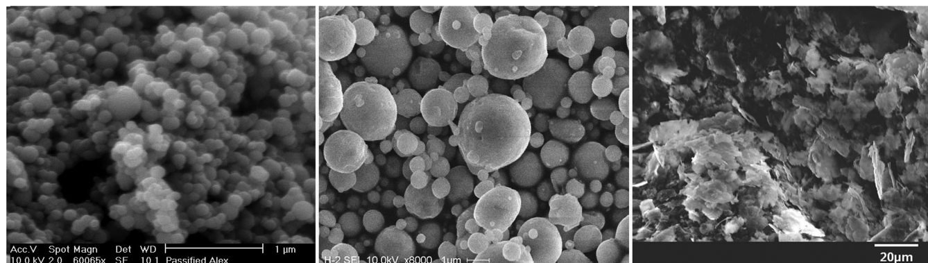
Fig. 1 SEM of Al particles. Left: Alex with a mean diameter of 100 nm; middle: atomized H-2 with a mean diameter of 1.6 \mu\text{m} by number; right: Silberline DF-1667 Al flakes.
